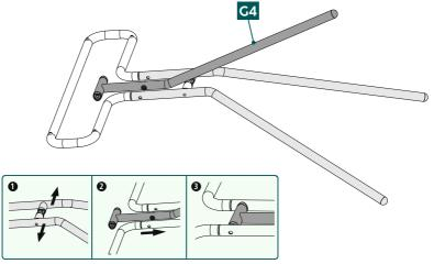
• In the next step, position the third support leg [G4] between [G2] and [G3] as shown above. Make sure that the screw and threaded holes are exactly on top of each other so that they can be screwed together in the next step.
