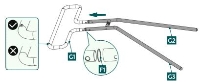
• First attach the two support legs [G3 and G2] together with the connecting rings [F1] to the mounting bracket. Ensure that the screws of the mounting bracket are positioned as shown above.
