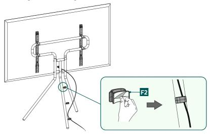
• Attach the supplied cable clips [F2] to the centre leg as shown in the illustration and then feed the cables through.
