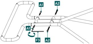
• Secure the support legs using screws [A1] in the upper area and [A2] screws in the lower area. Use the enclosed Allen key [F3] for installation.
