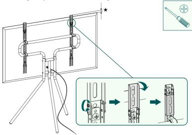
• Depending on the size of the mounted TV, the VESA arms may protrude beyond the TV. After removing the side screws, the VESA arms can be folded up or down as required.
