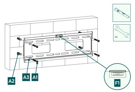
• Attach the wall bracket to the wall as shown above using the enclosed mounting material ([A2] plug, [A3] M8 washer, [A1] 8x60 mm screw and [F1] spirit level).
