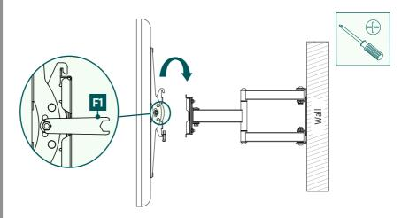
• Then fix the lateral fastening screws using the hexagon ring spanner included [F1].
