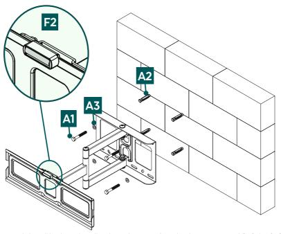
• Attach the wall bracket to the wall as shown above using the enclosed mounting material ([A2] plug, [A3] M8 washer, [A1] 8x60 mm screw and the [F2] spirit level).
