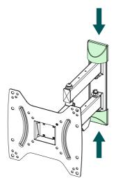
• Then attach the two enclosed covers to the bracket.
