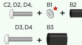
$\text{M8x50} + \text{ø8x5} = \text{M8x45 (D4)}$
