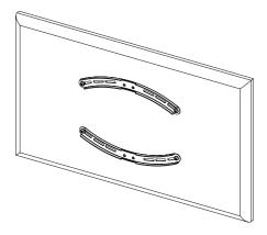
When positioning the VESA arms on the back of the TV, note the corresponding VESA mount. Depending on the VESA variant required, the VESA arms may need to be aligned differently. These are positioned either outwards (see 6.3.1) or inwards (see 6.3.2) in a curved manner.
