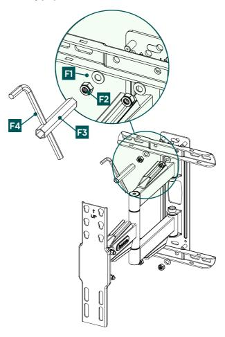
Mount the horizontal struts on the wall mounting plate as shown above. Note the combination of the flange nut [F2] and washer [F1] as listed above. Use the pipe socket spanner [F3] and Allen key [F4] included to secure them.
