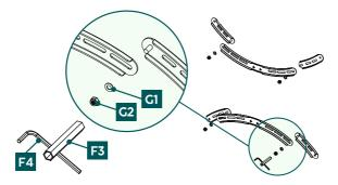
Fit the supplied VESA adapters on the left and right to the VESA arms using the washers [G1], screws [G2] and pipe socket spanner [F3] and Allen key [F4].
