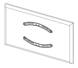
When positioning the VESA arms on the back of the TV, note the corresponding VESA mount. Depending on the VESA variant required, the VESA arms may need to be aligned differently. These are positioned either inwards (see 6.3.1) or outwards (6.3.2) in a curved manner.
