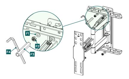
Mount the horizontal struts on the wall mounting plate as shown above. Note the combination of the flange nut [F2] and washer [F1] as listed above. Use the pipe socket spanner [F3] and Allen key [F4] included to secure them.
