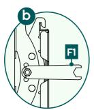
• Then fix the lateral fastening screws using the hexagon ring spanner [F1]).
