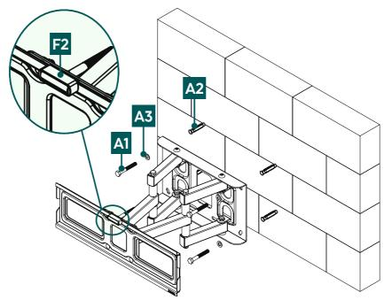
• Attach the wall bracket to the wall as shown above using the enclosed mounting material ([A2] plug, [A3] M8 washer, [A1] 8x60 mm screw and [F2] spirit level).
