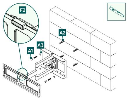
• Attach the wall bracket to the wall as shown above using the enclosed mounting material ([A2] plug, [A3] M8 washer, [A1] 6x55 mm screw and the [F2] spirit level).
