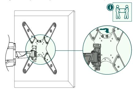
• Hang the TV with the mounted VESA plate on the wall bracket as shown above.
