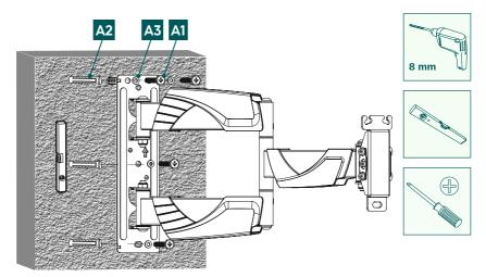
• Attach the wall bracket to the wall as shown above using the enclosed mounting material ([A2] plug, [A3] M6 washer, [A1] 6x55 mm screw).
