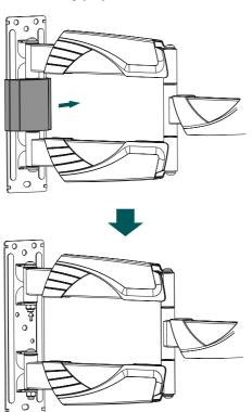
$\bullet$  Remove the centre cover from the wall plate.
