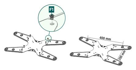
Mount the supplied adapter plates on the back of the VESA plate using screws [F1].
