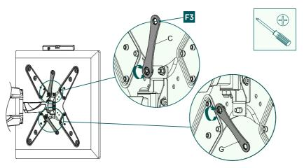
• Then tighten the fixing screws with the enclosed hexagon ring spanner [F3].
