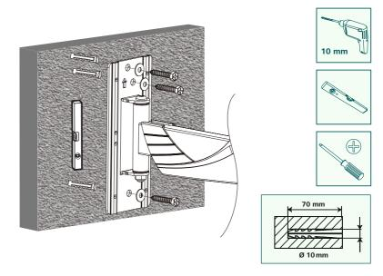
Attach the wall bracket as shown above using the enclosed mounting material ([A2] plugs, [A3] M8 washer, [A1] 8x60 mm screw) to the wall.
