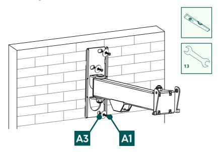
• Attach the wall bracket to the wall as shown above using the enclosed mounting material ([A2] plug, [A3] M8 washer, [A1] 8x60 mm screw).
