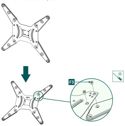
• Mount the supplied VESA adapters on the back of the VESA plate using screws [F3].
