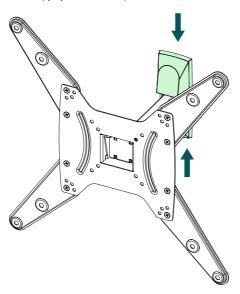
• Then attach the two enclosed covers to the bracket.
