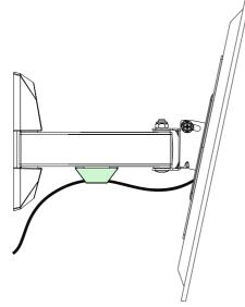
• Feed the cables through the cable manager.
