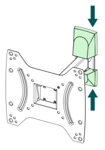
• Then attach the two enclosed covers to the bracket.
