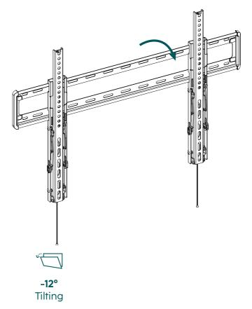
• No screws need to be loosened to adjust the tilt.
