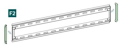
Attach the two enclosed covers [F2] to the bracket.
