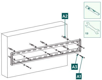
• Attach the wall bracket to the wall as shown above using the enclosed mounting material ([A2] plug, [A3] M8 washer, [A1] 8x60 mm screw and the [F4] spirit level).
