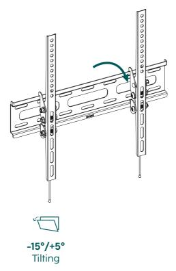
• To adjust the tilt angle, open the fastening screws at the side, set the required tilt, and then secure the screws in place again.
