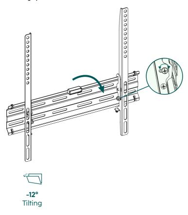
• To adjust the tilt angle, open the fastening screws at the side, set the required tilt, and then secure the screws in place again.
