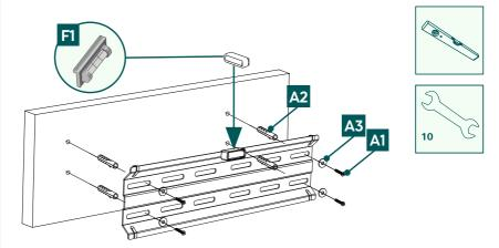
• Attach the wall bracket to the wall as shown above using the enclosed mounting material ([A2] plug, [A3] M6 washer, [A1] 6x50 mm screw and the [F1] spirit level).
