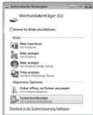
When you have chosen the command **Speed up my system**, the following property window appears. Please select the command **Use this device** in the tab ReadyBoost in order to activate the ReadyBoost function.
