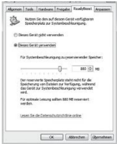
With the sliding regulator you determine how much memory you want to use for the ReadyBoost function. The system reserves the selected capacity as ReadyBoost.sfcache; the FlashPen "Steady" can only be used as mass storage medium again if ReadyBoost is deactivated for the stick.
