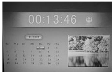
**Settings:** The calendar and time are set as follows. Select “Setup” from the main menu and confirm with “Enter” to open the setup menu. Under the setup time “Time”, you can set the current time and date. Select the year, month, day Hour and minute and change the value using the “▲▼” buttons. Confirm your selection using the “Enter” button.
