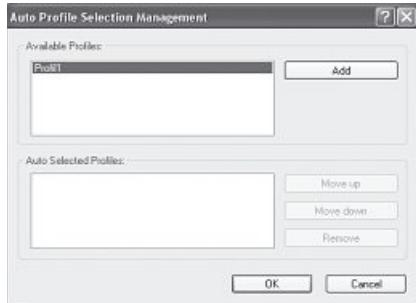
Select the required profile in the list of the **Available profiles**. Click **Add**. The profile select is then displayed in the list of **Automatically selected profiles**. That means that this profile is run automatically, e.g. after a restart. If there is more than one profile in this list, you can set the required sequence with the **Move up** and **Move down** buttons. The **Remove** button allows you to delete a profile from the list.
