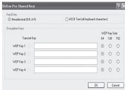
The entries you make here must be exactly the same as the encryption data in the target network, i.e. in the wireless LAN router/access point in infrastructure mode and as all client WLAN devices in ad-hoc mode.
