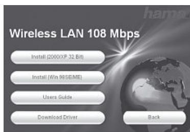
To continue installation, click **Install (2000/XP 32 bit)** if you use Windows® 2000 or XP as an operating system. The stick can also be used with restricted functions for the Win 98/ME operating systems. With these operating systems, the Extended Range (XR)TM function is not available and the software is in English only. Click **Install (Win 98/ME)** if you use Windows® 98 or Windows® ME.
