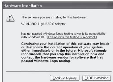
This only means that the test has not been performed. The stability and function of the driver was tested thoroughly before delivery. The qualification of the drivers by Hama means that new versions can be used far earlier and do not have to wait for the Windows® logo test. Click **Continue installation** to confirm the message.
