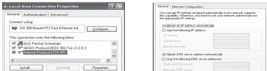
Select **Obtain an IP address automatically** and **Obtain DNS server address automatically**, if there is a DHCP server in your network! Confirm by clicking **OK**, and again in the subsequent window. Your PC is now configured such that the router assigns the IP address automatically.
