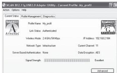
The signal strength and corresponding information on your configuration should now be displayed here. You can now close the configuration tool. The activated profile is run automatically after a restart.
