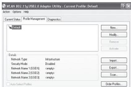
When configuring your USB stick, it is useful to create a profile. A profile serves to save various settings for a connection under a certain name. For example, if you want to connect to various wireless networks, you can save the settings for the networks in profiles, which allows you to change the configuration quickly.
