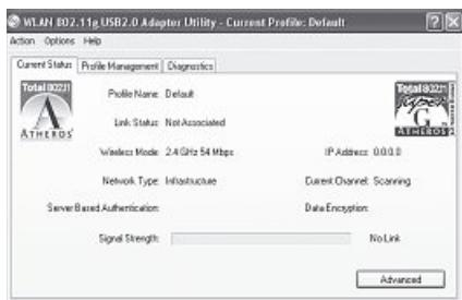
This view gives you information on various settings of your wireless LAN. If the target network to be connected is not encrypted, the WLAN device may already have automatically connected to an available network. If this is the case, the signal strength display at the bottom of the screen shows a signal.
