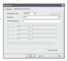
To use **WPA2 encryption**, select **WPA2-PSK** under Authentication type and **AES** under Encryption. Now enter the code used in the WPA preshared key field.
