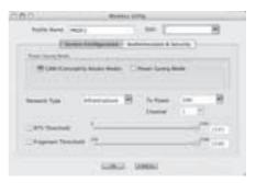
The settings for TX Power, Channel, RTS Threshold and Fragment Threshold can be left at the default settings.
