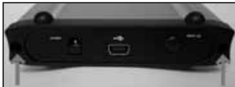
Attach the rear of the housing with the sockets provided to the connection row of the hard drive. "Pin1" is marked on both the rear of the housing and on the hard drive.
