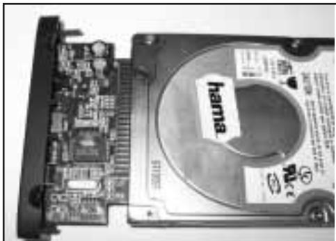
After you have connected the hard drive and the rear of the housing correctly, insert the hard drive with the rear of the housing into the aluminium housing.
