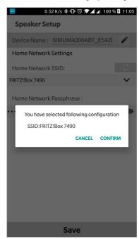
The loudspeaker now connects to the network. After successful connection, "Loudspeaker configured successfully" appears on the smartphone.
