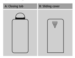
Insert the batteries provided, making sure you match the polarities correctly. The correct polarity is indicated by the plus and minus symbols in the battery compartment.
