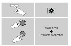
• Then select the YES button by turning [ENTER/ **NAVIGATE**], and confirm termination of the Bluetooth connection by pressing [ENTER/NAVIGATE].
