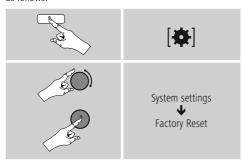
Confirm the following prompt with **YES** to reset the radio to the factory default settings. All settings made previously are deleted.
