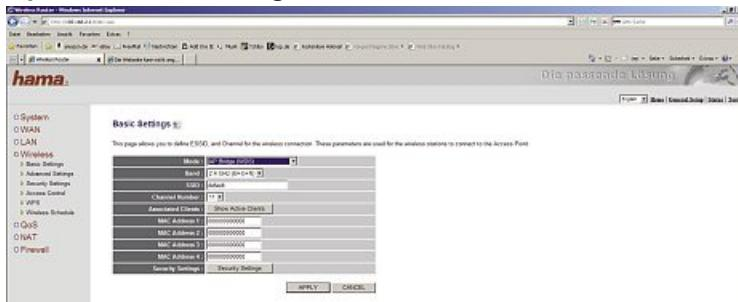
WDS (Wireless Distribution System) is the term for the wireless connection between several access points. In addition, it permits the login of clients that other bridge operating modes do not allow. For each additional access point, the bandwidth of the network is halved because the packages have to be transmitted double.
