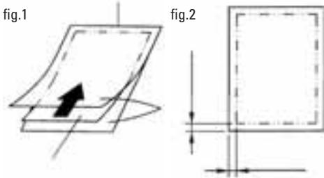
4. When the ready light is completely white, insert the laminating pouch squarely and centrally (with the sealed side first) into the front of the laminator.
