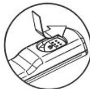
For long exposures or continuous shooting, press the release button completely and slide it in the direction of the arrow. This locks the button in the depressed position. To release, slide the button back to its original position.
