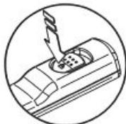
The release button can be pressed halfway or all the way. Pressing it halfway activates the autofocus and sets the shutter speed and aperture settings. Pressing it completely takes the picture.
