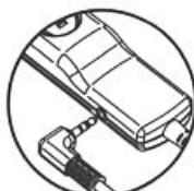
Plug the synchro-cable into synchro-socket of the remote cord to make two cameras take picture simultaneously. (Only for special model.)
